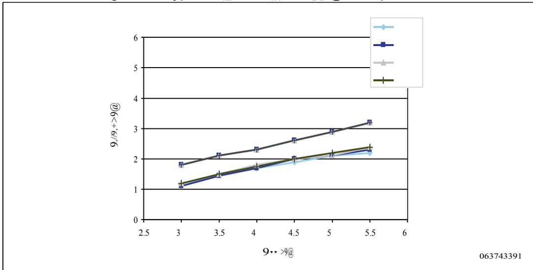
Figure 21. Typical pull-up resistance vs  $V_{DD}$  @ 4 temperatures
