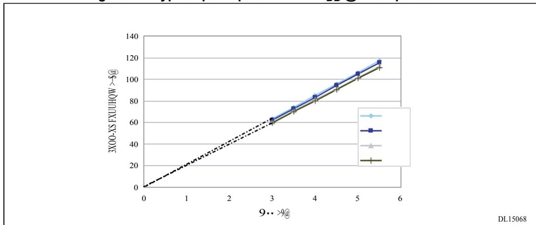
1. The pull-up is a pure resistor (slope goes through 0).
