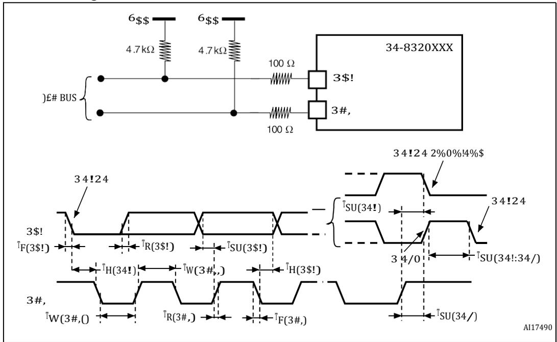
1. Measurement points are made at CMOS levels:  $0.3 \times V_{DD}$  and  $0.7 \times V_{DD}$
