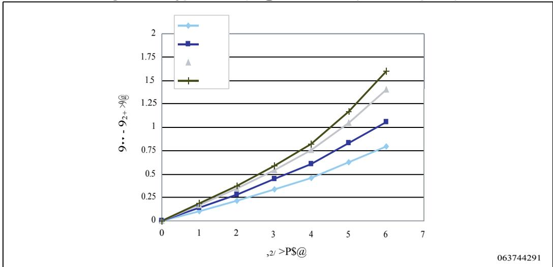
Figure 31. Typ.  $V_{DD} - V_{OH}$  @  $V_{DD} = 5\text{ V}$  (high sink ports)
