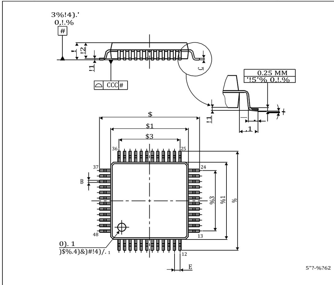
Table 54. LQFP48 - 48-pin, 7x 7 mm low-profile quad flat package mechanical
